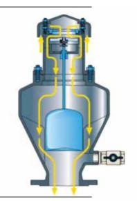
B - Discharge of large volumes of air during pipe filling it is necessary to discharge as much air as the water flowing in.
