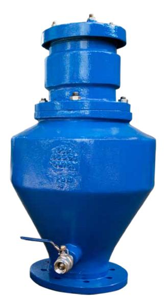
GCF sewage air valve series 6500 Are Hydro mechanical devices designed to automatically release or admit air during pipeline filling, draining, or operation of a water pipeline or system. The safe operation and efficiency of a pipeline are dependent on the continual removal of air from the pipeline.
