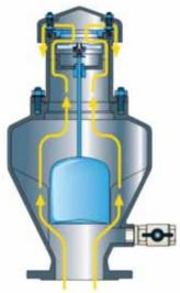
C - Air release during working conditions during operation, an air pocket accumulates in the upper part of the valve body; little by little it is compressed and released automatically.
